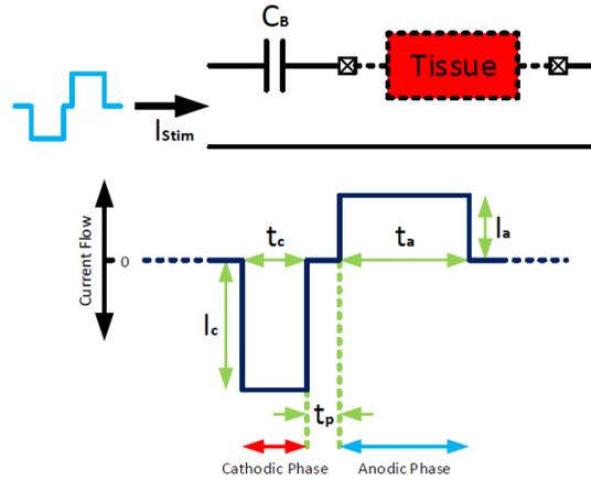
Figure 4.3: Biphasic stimulation (assuming blocking capacitor is used).
